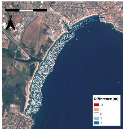
Example of validation for Sentinel-2 derived bathymetry (2017)
